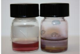
Figure 2.3: on the left, red colloidal suspension of  $\sim$ 7nm nanoparticles, on the right the suspension after some time. Note how the violet-blue aggregated particle fill the top part of the solvent.
