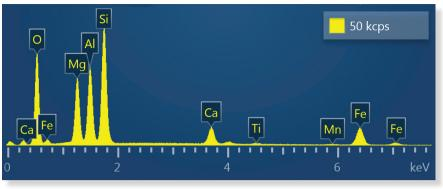
Almandine garnet spectra collected at different beam currents: resolution and peak position stay constant over a large count range.
